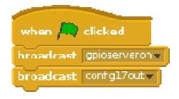
• From this point on, you can control your LED using two broadcasts: "GPIO17ON" to turn it on and "GPIO17OFF" to turn it off. Using these two messages and some pauses, you can make an LED flash continuously.
